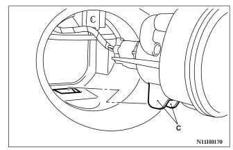
4. When mounting the light unit, align the pin (C) on the light unit with the hole in the body.
